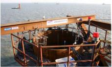
Top of pile instrumentation and reference beam as test on W8 was in progress
